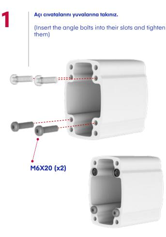
$4x \qquad 4x \qquad M6 \times 30$   $2x \qquad M6 \times 20$   $4x \qquad 0 \qquad J6.4$   $1x \qquad M5 \times 8$   $2x \qquad 2x \qquad 2x \qquad 1x$   $2x \qquad 1x \qquad 1x \qquad 1x$
