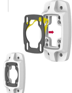
(Insert the profile into the coupling as shown in the picture below)
